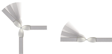
Images showing how individual screens can be ganged together in various combinations
